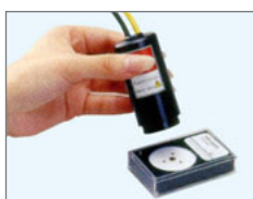
A probe checker controls the probe before measuring
