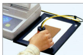
To measure just hold the probe perpendicularly to the sample
